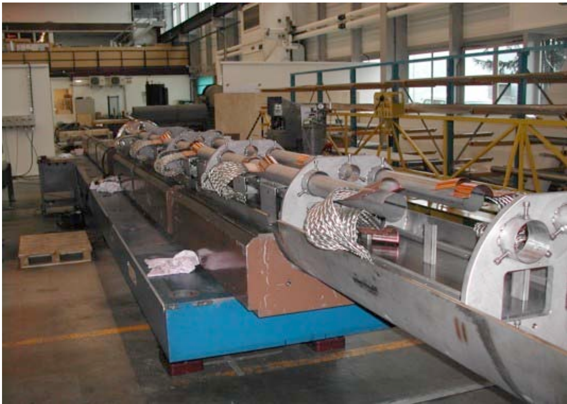
Figure 4.1. The 420m interconnection cryostat at LHC start-up
